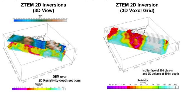
Figure 3: 2D Resistivity inversion of ZTEM results over Pebble porphyry deposit showing: a) 2D cross-sections arranged in 3D view with DEM elevation model (left) and b) 2D results combined in 3D voxel grid volume showing 100 ohm-m iso-surface (right).
