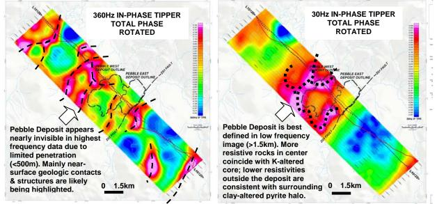
**Figure 2:** ZTEM Tipper AFMAG field results shown in plan as grid contours of 90-degree Total Phase-Rotated (TPR) In-Phase component at: a) 360Hz high frequency showing shallower penetration (left) and .b) 30Hz low frequency showing deeper penetration (right).
