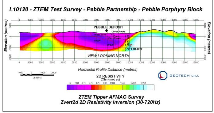
Figure 1: 2D Resistivity cross-section over center of Pebble porphyry deposit from Zvert2d inversion of ZTEM In-line (Z/X) tipper data.
