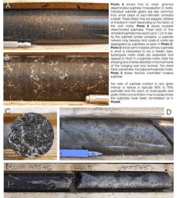
Figure 4: Slide showing texture of sulphides in Axis Lake diamond drill core (after Vivian and Lo, 2007).
