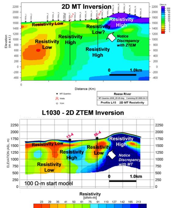
Figure 9: 2D Inversion of MT Line L15 (above) and ZTEM Line 1030 (below). Notice discrepancy below well 56-4.
