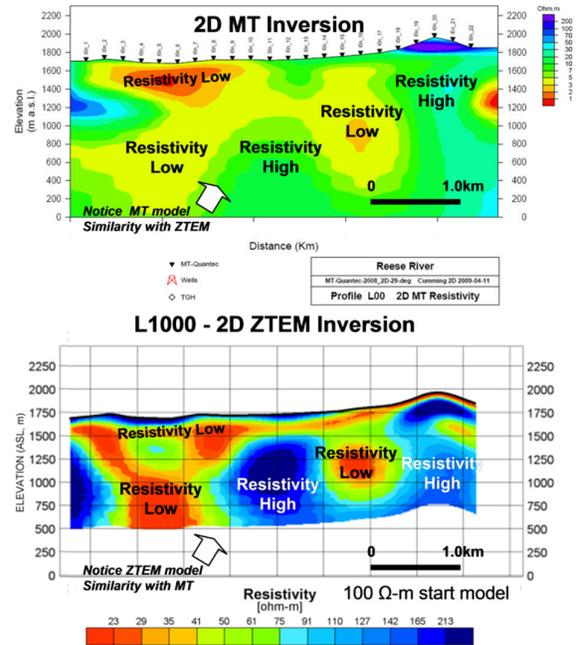
Figure 8: 2D Inversion of Ground MT Line LO (above) and ZTEM Line 1000 (Below). Notice MT similarity to ZTEM.
