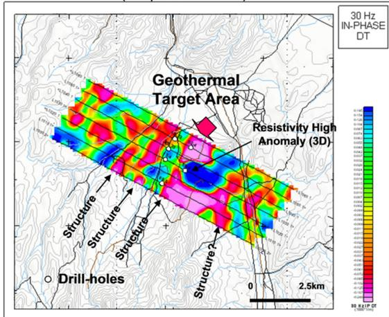
Figure 7: ZTEM 30 Hz In-phase Total Divergence (DT).
