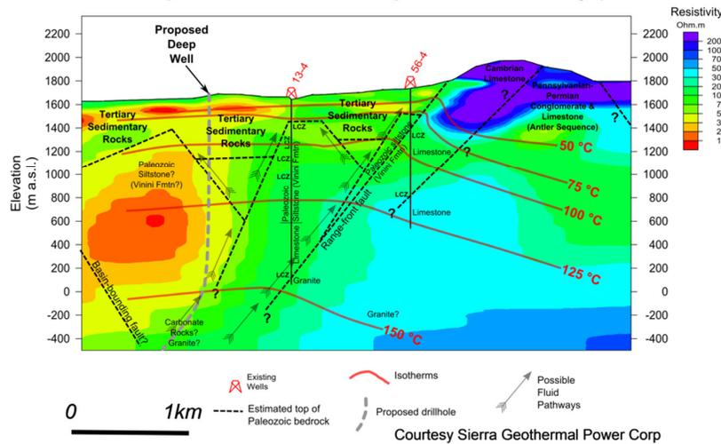
Figure 4: Cross-section through the Reese River prospect showing 2D MT resistivity inversion, depth to bedrock (estimated from gravity, geology and borehole data), temperature isotherms from boreholes, subsurface geology, existing wells and possible fluid pathways (revised after Witter et al., 2009).
