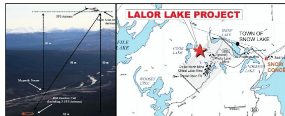
Figure 1:a) ZTEM helicopter receiver system (left) and b) Lalor Lake location with ZTEM flight lines (right – modified after Blakley, 2008).
