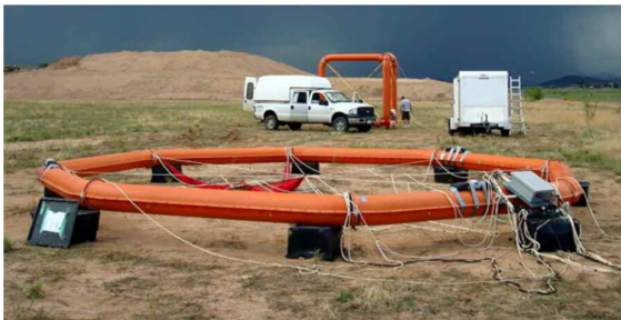
Figure 1: ZTEM Hz Receiver Coil (foreground) and Hx-Hy Reference Coils (background).
