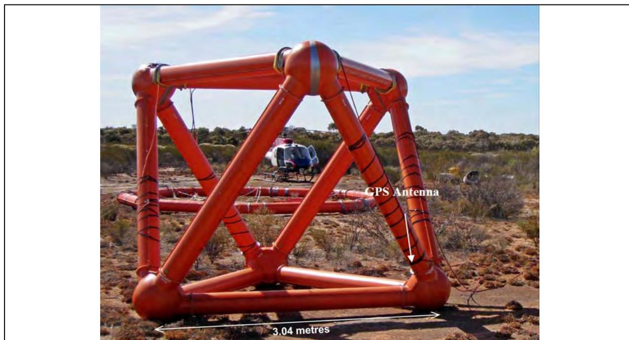
Figure 3. ZTEM and AirMt base station sensor.
