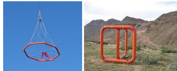
Figure 1: (Left) Z-TEM receiver coil in survey, (right) base station setup while on survey.
