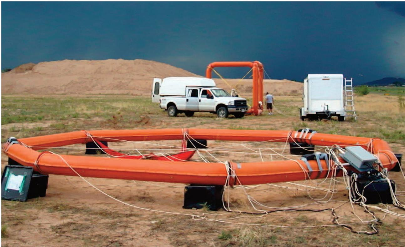
**Figure 1:** *ZTEM Hz Receiver Coil and Hx-Hy Reference Coils*
