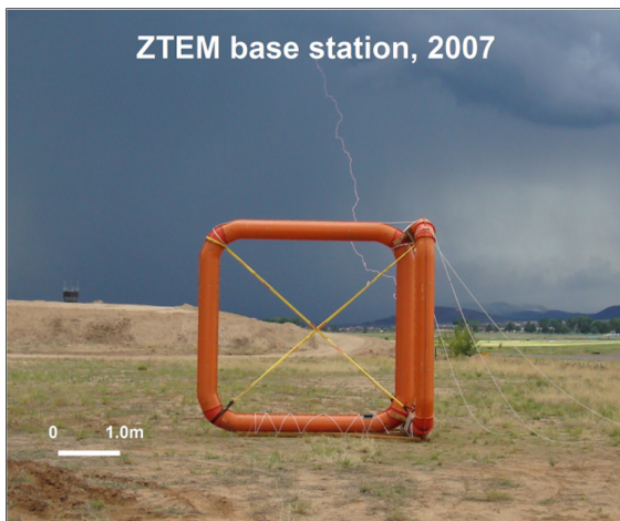
Figure 4: ZTEM base-station receiver in 2007 field surveys in Arizona USA (after Lo and Kuzmin, 2008).
