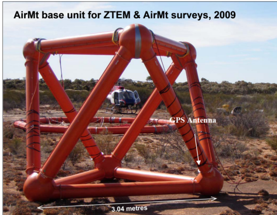
Figure 7: AirMt sensor, deployed as ZTEM and AirMt base-stations, during field trials in Western Australia in 2009.
