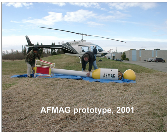
Figure 1: Airborne AFMAG prototype, in early 2001, with nose-cone removed (after Kuzmin et al., 2005).
