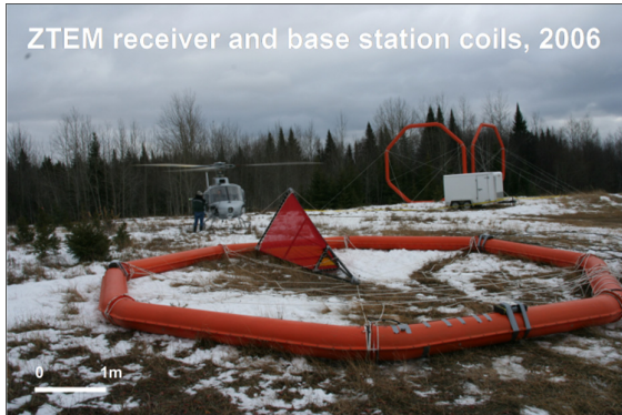
Figure 3: ZTEM z-axis receiver (foreground) and ground-based prototype reference coils (background) from field tests in northern Ontario CAN in 2006 (after Thompson et al., 2007).
