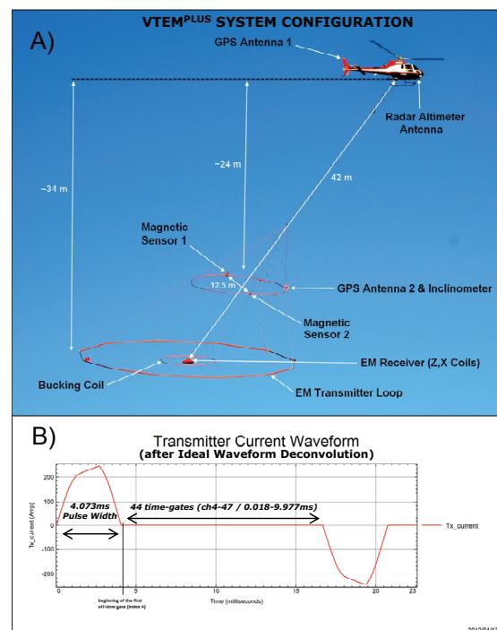
Figure 1: A) VTEM<sup>PLUS</sup> helicopter EM system and b) transmitter current waveform (after ideal waveform deconvolution).
