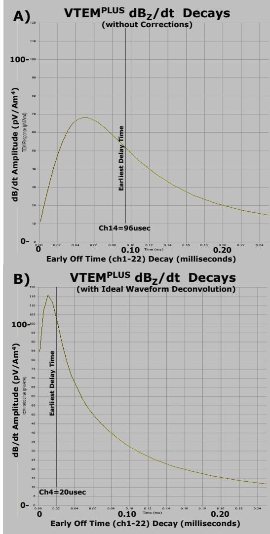
Figure 2: Spiritwood early off-time VTEM  $\text{dB}_z/\text{dt}$  decays: A) before correction and B) after system response correction & ideal waveform deconvolution (Legault et al., 2012).
