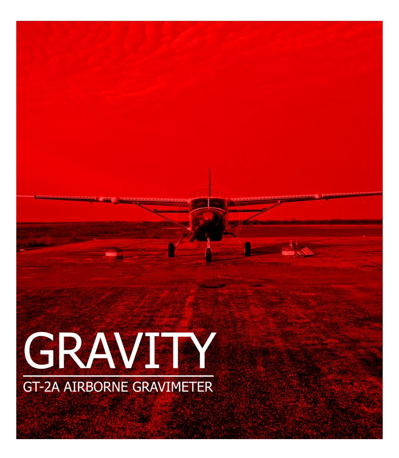
Earth's gravitational field is not uniform; the denser the rock, the greater the gravitational field. As a result, very precise measurements can detect critical variations in rock density. Geotech has flown more than one million line-kilometres measuring minute gravitational field differences.
