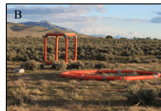
Figure 1. (A) ZTEM base station (square with a side length of 3.5 m) in foreground with lightning strike in the background. (B) ZTEM airborne receiver (circle with a diameter of 7.2 m) in foreground, ZTEM base station in the background.
