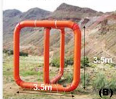
Figure 5: a) Magnetotelluric skin depth chart (left) showing the calculated ZTEM™ AFMAG minimum to maximum depth investigation versus earth resistivity; b) ZTEM™ Hx-Hy base station coils (center), c) ZTEM Hz receiver (right).
